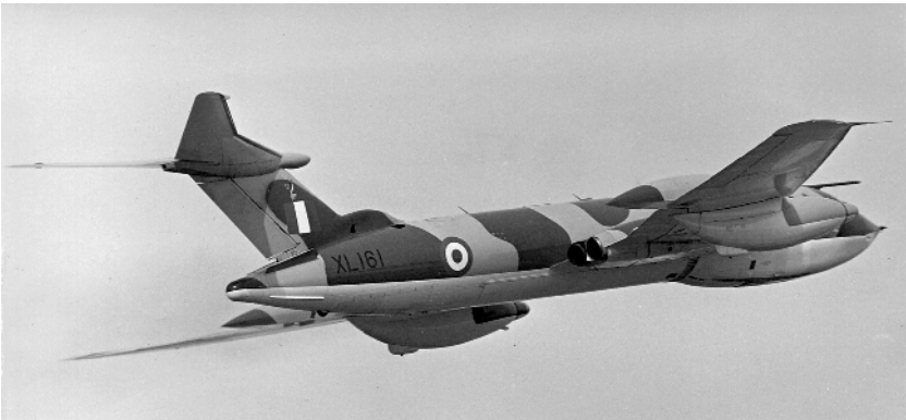
A Victor B.2(SR) of No 543 Sqn. Note that both underwing fuel tanks have had ‘pudding basins’ added to permit atmospheric sampling for the analysis of nuclear fallout.
