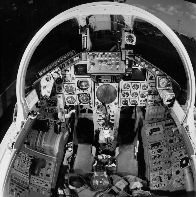
Front cockpit of an early production Tornado GR 1
