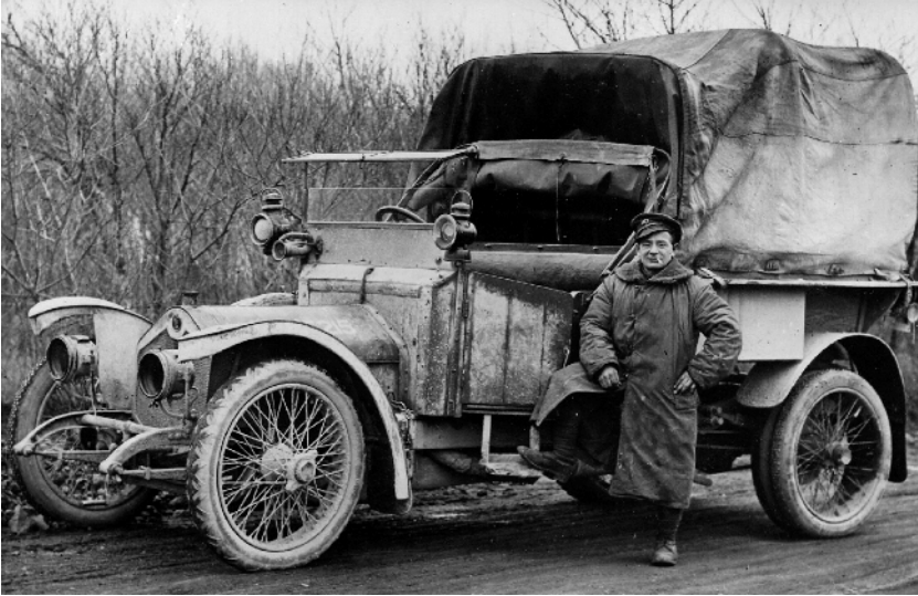
Representative of the kinds of vehicles used by the RFC/RAF to move supplies around – a 25hp Crossley tender.
