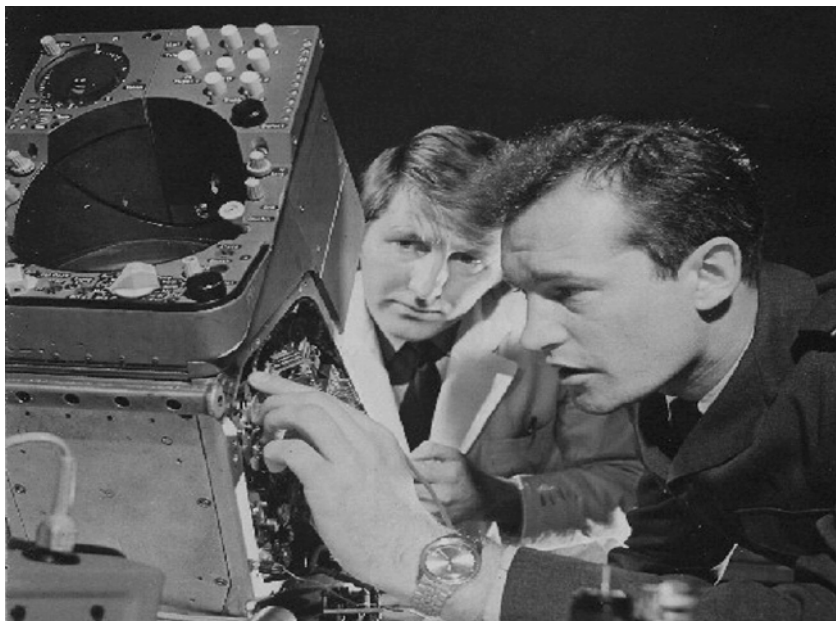
Fg Off O'Reilly investigates the innards of a Harrier's moving map display under the anxious gaze of an instrument fitter.
