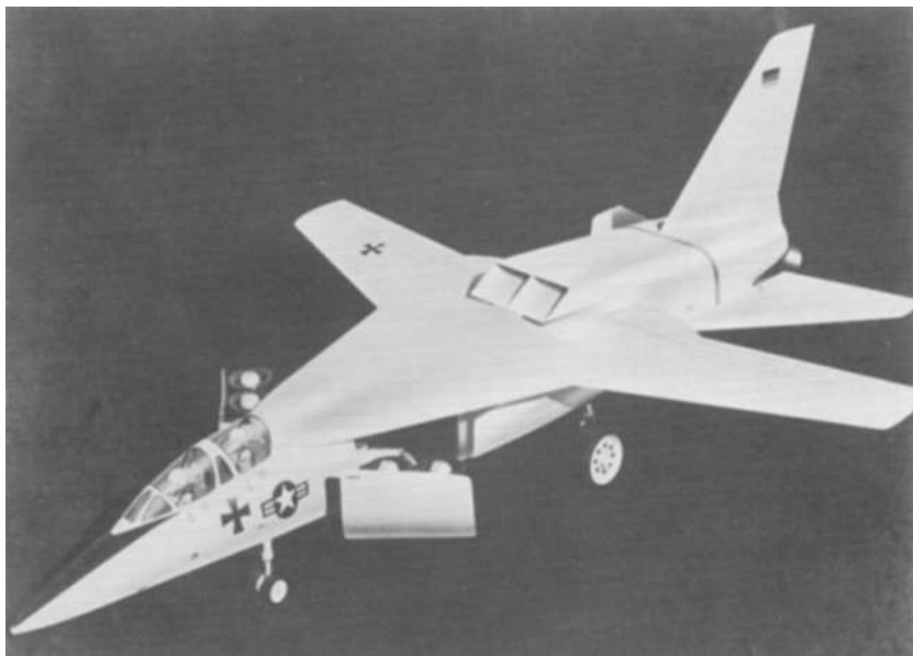
Joint US/FRG project for a V/STOL strike fighter employing retractable and vectorable lift engines and variable geometry wings.
