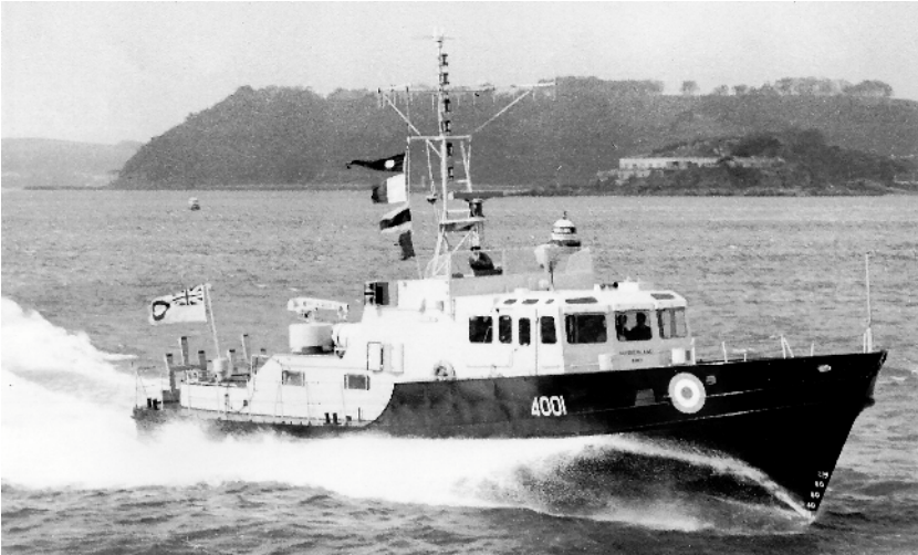
The 60-ton HMAFV Sunderland at speed, a little over 20 kts, off Mount Batten. (Donald Smith)
