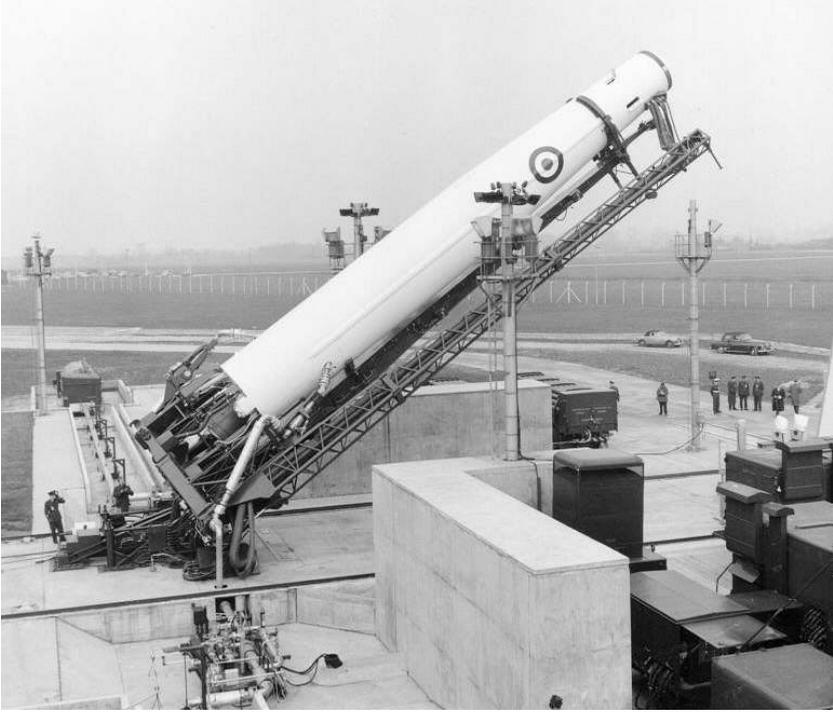
*A Thor being erected during the transition from a readiness state of T-15 to T-8.*
