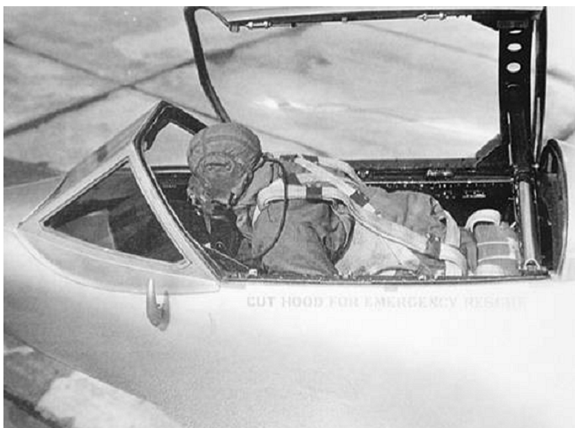
Above – the Reid and Sigrist RS3 Desford, seen here after conversion to become the prone-pilot RS4 Bobsleigh, which was used for trials work from 1951, supplemented from 1954 by a modified Meteor (below).
