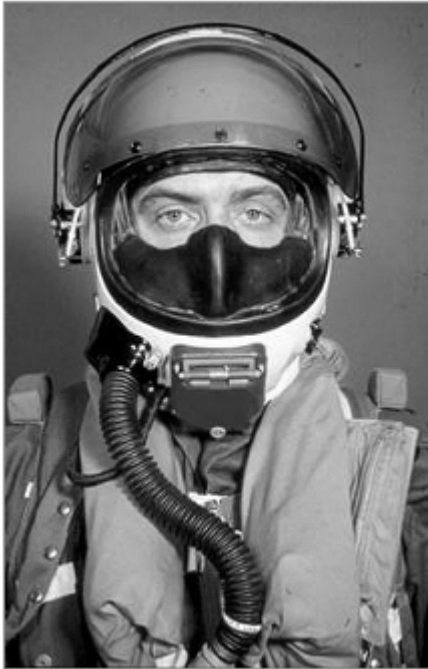
Partial Pressure Helmet and Pressure Jerkin developed by IAM for high altitude protection in the Lightning.
