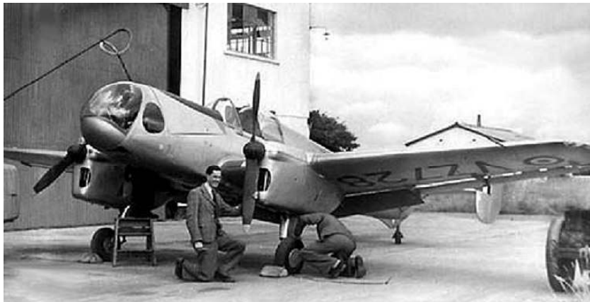
Above – the Reid and Sigrist RS3 Desford, seen here after conversion to become the prone-pilot RS4 Bobsleigh, which was used for trials work from 1951, supplemented from 1954 by a modified Meteor (below).
