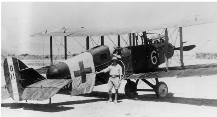
Well- known picture of one of the DH 9s modified for use as an air ambulances during the Somaliland expedition of 1919.
