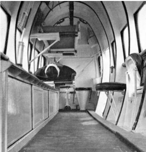
Above, a Vernon Ambulance, J7143, of No 45 Sqn and (left) its interior.
