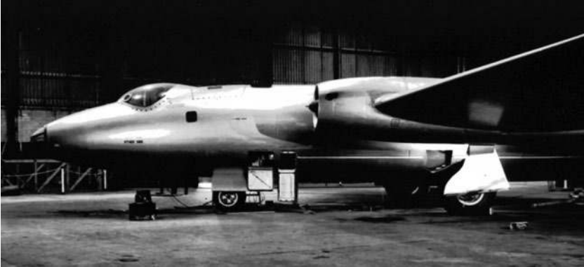
PR3, WH726, having its LOROP 'Bomb Camera' installed at Hanscom AFB in 1954 in preparation for Op ROBIN.
