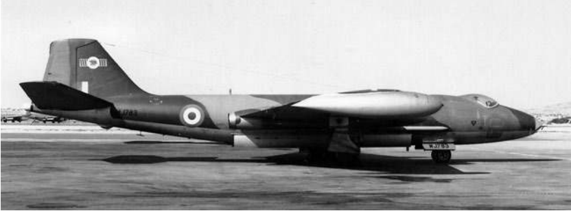
One of No 249 Sqn's Canberra B16s displaying its BLUE SHADOW aerial on the starboard side of the forward fuselage, the only external feature that distinguished it from a B 15. (MAP)
