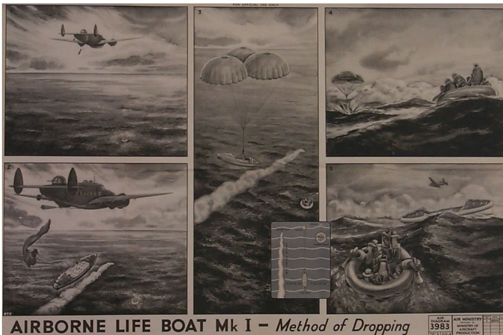
Diagram showing the deployment of an airborne lifeboat. These were used by Coastal Command during the Second World War to rescue downed aircrew.
