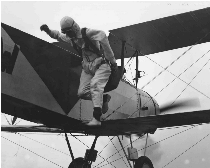
Parachute jump from a biplane. Notice that the parachute is strapped to the parachutists bottom rather than worn as a rucksack as today.
