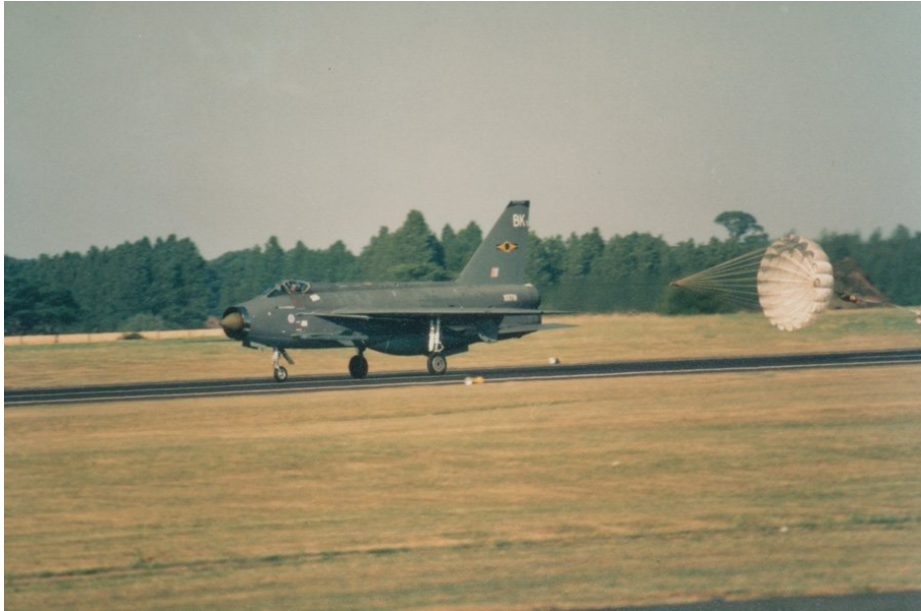
Parachute being used to slow down an English Electric Lightning aircraft upon landing.
