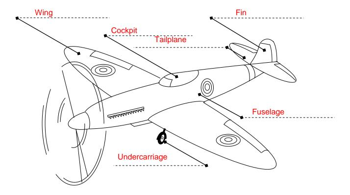
The large model Spitfire in the Aeronauts gallery will help you find out about the different parts of an aeroplane and how they work.
