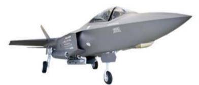
The **F-35** is a single-seater, supersonic stealth aircraft which has been designed to fly at speeds of over 1,000 miles per hour.
