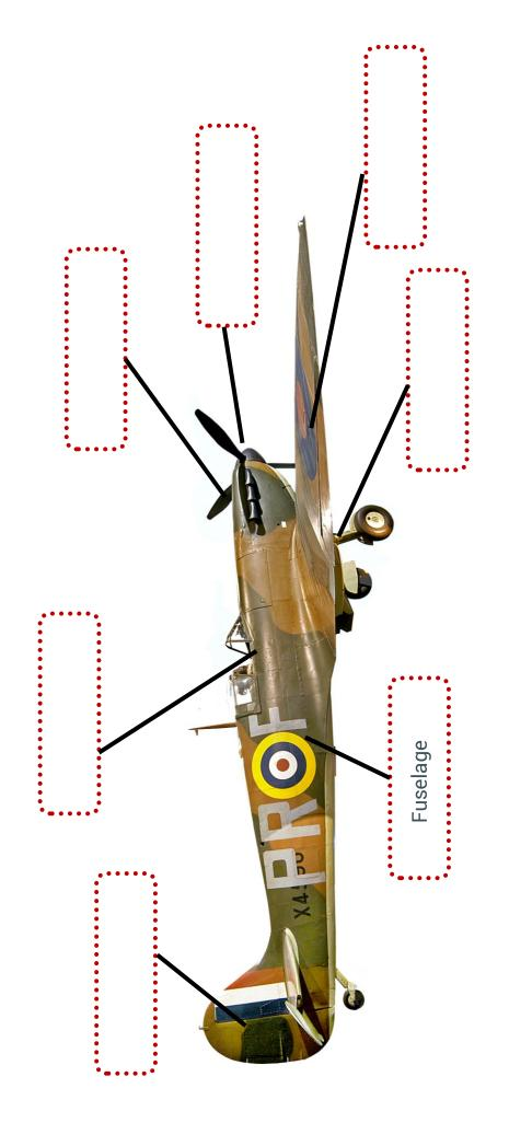
Propeller Wing Undercarriage Nose Cockpit Tail **Fuselage**
