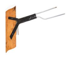
It is fundamentally important to know an aircraft's speed through the air. This can be achieved by the use of a Pressure Head. The difference between the static pressure of the upper vent and the dynamic pressure of the airflow entering the lower tube is transmitted and displayed on the scale of an Air Speed Indicator.
