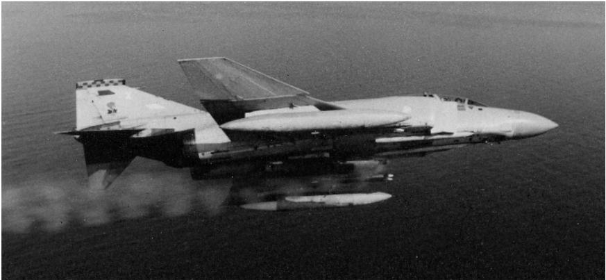
*A Phantom FGR2 of No 92 Sqn firing its pod-mounted SUU-23 Vulcan cannon*
