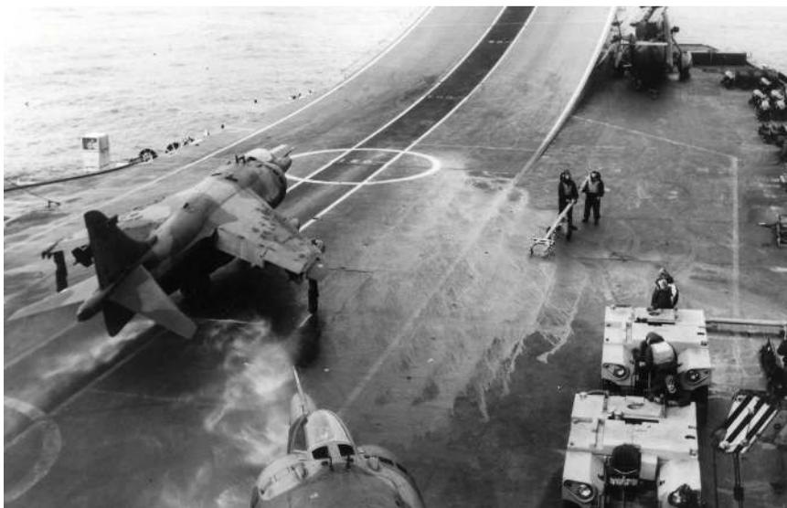
*In seaborne operations, V/STOL aircraft may be more tolerant of adverse weather conditions than conventional types. These Harriers of No 1 Sqn are preparing to launch from HMS Hermes.*
