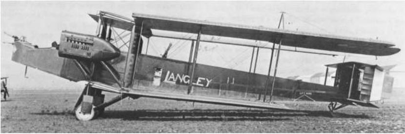
*The plan to produce Handley-Pages in the USA failed to bear fruit before the Armistice. This one, B9449, is the O/100 that was modified in the UK before being shipped across the Atlantic to serve as the pattern airframe for the Liberty-powered American-built O/400.*
