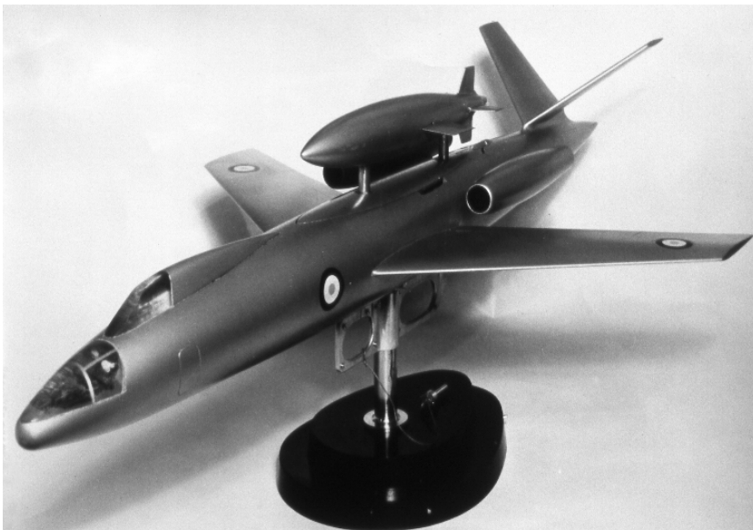
A model of the Type 186. The weapon, normally semi-recessed into the upper surface of the fuselage, is seen here extended, with its wings deployed, as it would have appeared immediately prior to ignition and launch.
