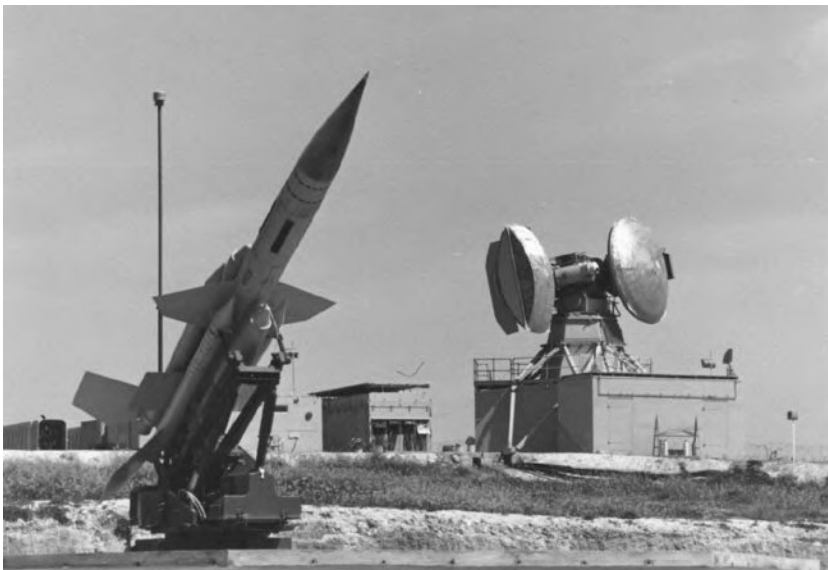
A Bloodhound II of No 112 Sqn at Paramali in Cyprus with a massive Type 87 BLUE ANCHOR radar in the background. (Stuart Baines)
