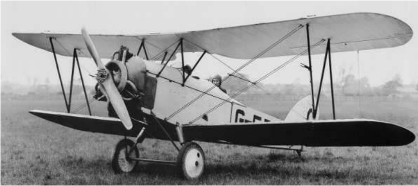
The Bristol Type 83 Lucifer, also known as the PTM (Primary Training Machine), six of which were built for the Reserve Flying School; this one, G-EBFZ, was in use from 1923 to 1931.
