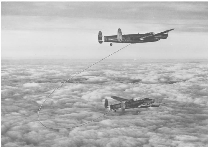
*Four of the eleven Lancasters allotted for wartime development were used for civil trials during 1946-47. Here, Lancaster tanker G-AHJW (ED866) refuels Lancaster receiver G-AHJU (LM681). FRL photo, neg. 167.*
