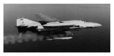
A Phantom FGR2 of No 92 Sqn firing its pod-mounted SUU-23 Vulcan cannon
