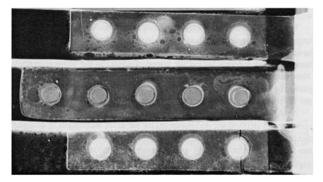
X-ray of one of the fifty-two three-fingered retaining brackets which secured the Vulcan's rear pressure bulkhead; the right hand bolthole of the lower bracket has failed.
