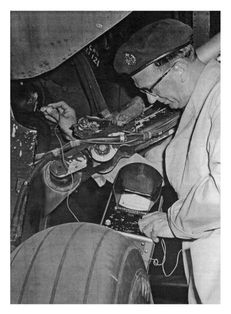
Carrying out an ultrasonic inspection on the undercarriage of a Canberra.
