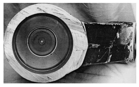
Section through a Canberra oleo showing a crack revealed by NDT.
