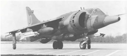
The Harrier's potential as an air defence fighter was enhanced by arming it with the AIM-9 Sidewinder.
