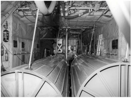
The range capability of the Hercules was increased, initially, as here, by the installation of auxiliary fuel tanks in the hold and, ultimately, by the provision of an AAR capability.
