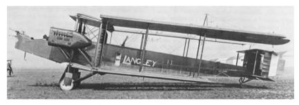
The plan to produce Handley-Pages in the USA failed to bear fruit before the Armistice. This one, B9449, is the O/100 that was modified in the UK before being shipped across the Atlantic to serve as the pattern airframe for the Liberty-powered American-built O/400.
