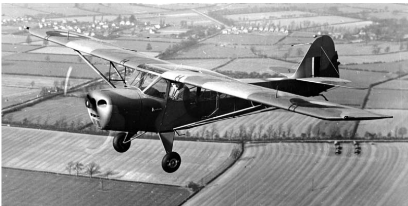
The Auster IV was characterised by its distinctive flat-four Lycoming.
